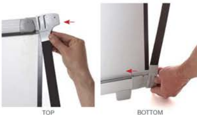
9 Slide in the top and bottom graphic joint from the side and mount the magnetic tape on the sides where you want to attach the Flex-Link graphic panel.
