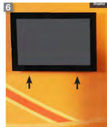
Lock the LCD with the two screws in the bottom of the screen rails!
